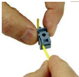
Figure A: Hold the cord clip so the two parts separate
