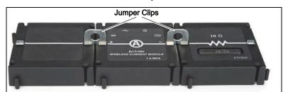
Usage: Use Jumper Clips to connect the Current Sensor Module as part of a circuit of other modules to measure the current through the circuit.
