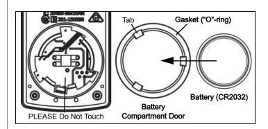
Remove the used battery from the Battery Compartment Door and replace it with a new identical type battery. *Note that the battery is held in place by the small tabs on the door.* The side of the battery with the "+" on it should be against the door.
